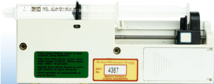
FIGURE 2.1 A battery-driven chemotherapy pump (Courtesy of Mr Simon Glazebrook, New Cross Hospital, Wolverhampton)
