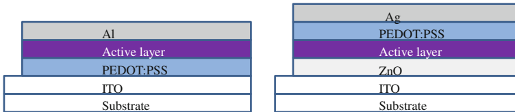
Fig. 2 Illustration of OPV devices, normal structure ( left ) and inverted ( right )
