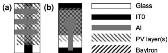
Fig. 7 Two common layouts for OPV devices with unpatterned PEDOT:PSS (Baytron) and photoactive layers: a In devices with the crosses layout, the Al electrode overlaps with the photoactive and PEDOT:PSS layers outside the patterned ITO region, b in this layout, outside the nominal area, the photoactive layer is in contact with unpatterned PEDOT:PSS/ITO only. Reproduced with permission from Cravino et al. [108], Copyright Wiley-VCH Verlag GmbH&Co. KGaA
