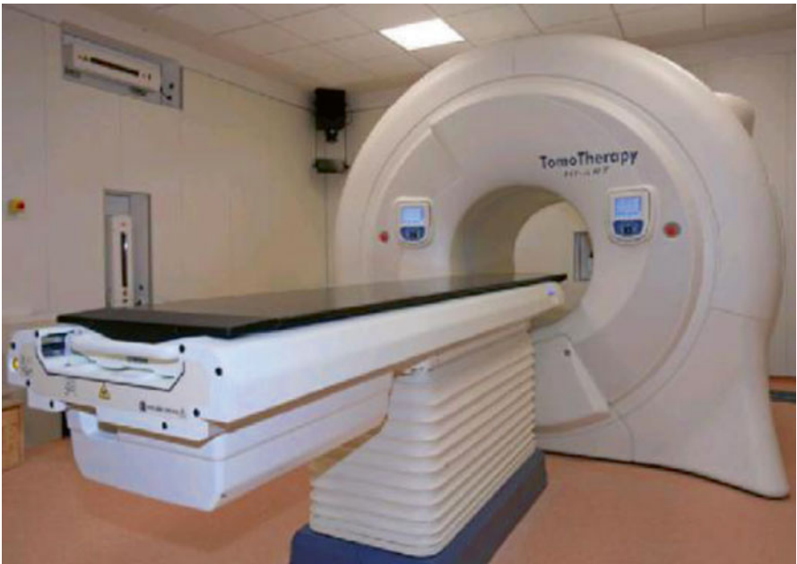
Fig. 3.4 Tomotherapy HDA, where the linac is mounted on the CT-like gantry and rotates through a full circle
