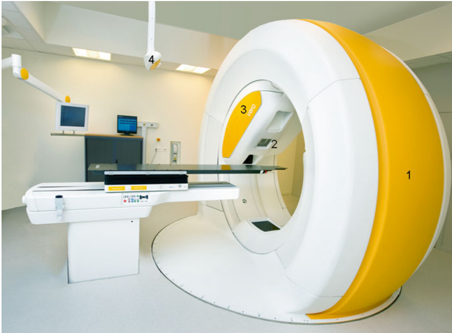
Fig. 3.5 The Vero SBRT System’s exterior view. The O-ring (labeled as “1”) is skewed in the counterclockwise direction. The ring can rotate over \pm 60^\circ . Label “2” indicates dynamic MLC, in both sides are two X-ray source. Label “3” indicates the gumbal for iso-center calibration and tumor chasing. Label “4” indicates the integrated real-time patient monitor
