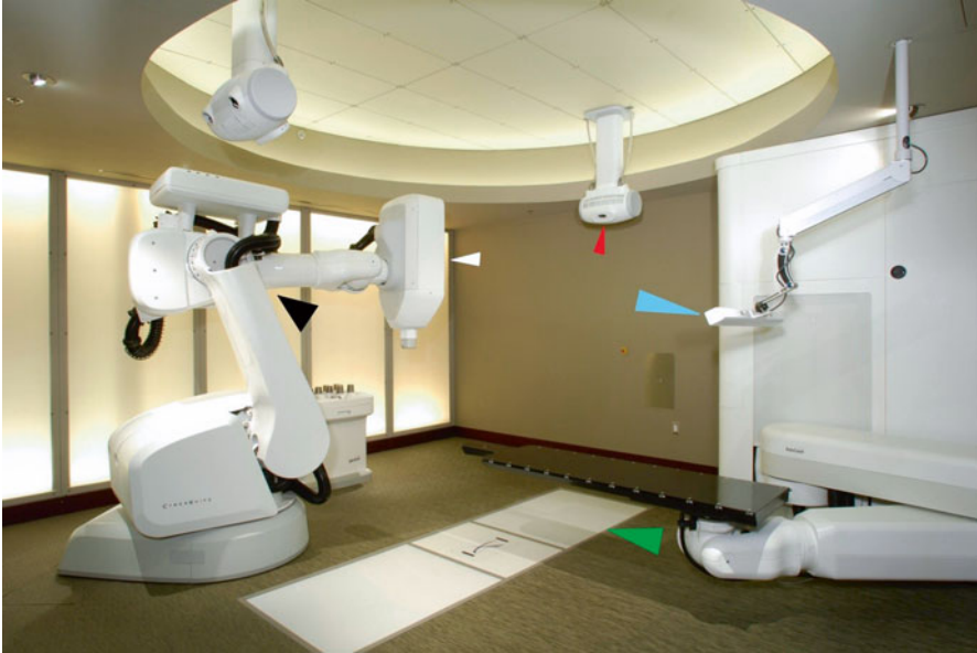
Fig. 8.2 The CyberKnife. White arrow , linear accelerator; black arrow , robot; red arrow , one of the 2 X-ray tubes; green arrow , one of the 2 flat panels; blue arrow , Synchrony camera
