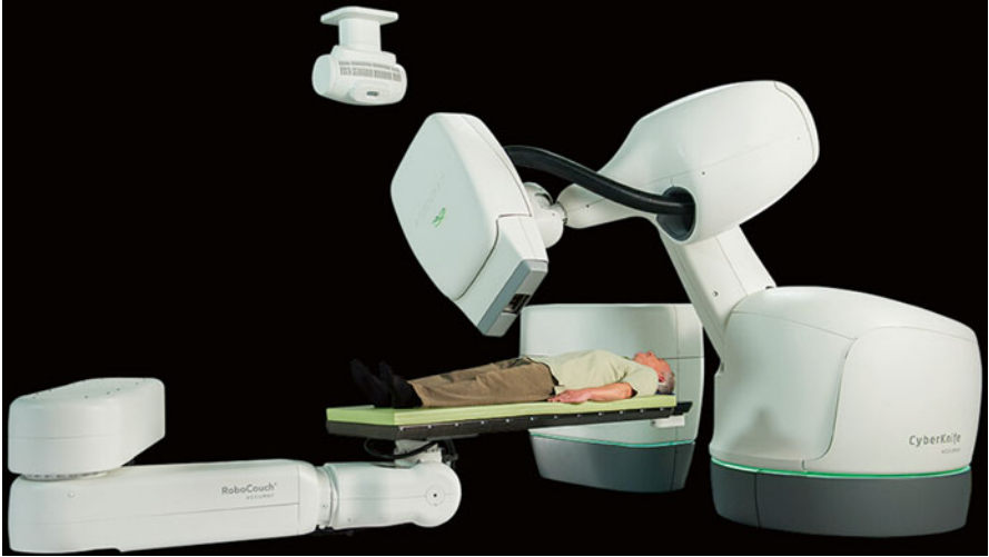
Fig. 3.3 A CyberKnife M6 system, where a robotic controlled linac, two X-ray sources, an optical monitor (on the left side ) and a couch are shown
