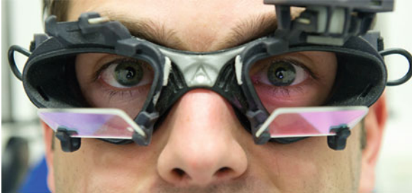
Fig. 1.19 Video-oculography (VOG) performed with a mask attached to the head in which a camera is integrated. An infrared headlight built into the mask also allows measurement of eye movements in complete darkness. The eye movements are shown online by means of a video-oculography program that continuously calculates the eye movements. Three-dimensional recordings can also be made by analyzing the movements of the picture of the iris
