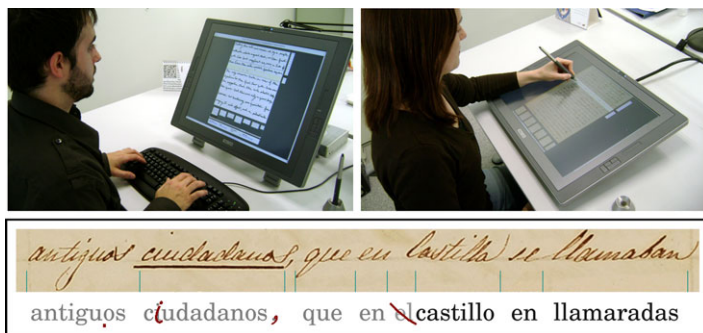
Fig. 3.5 Top : illustrations of CATTI multimodal user-interaction using keyboard and electronic-pen, respectively, on a touch-screen device. Bottom : page fragment showing a line image being processed, with a partially corrected system suggestion (in grey and black roman font) and the (previous) corrections made by the user through pen strokes and handwriting input marked in bold red
