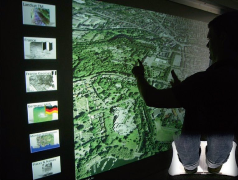
Fig. 16.3 User is interacting with both hands and feet with a virtual globe. The user is interacting with a large size multi-touch wall while standing on a Wii balance board
