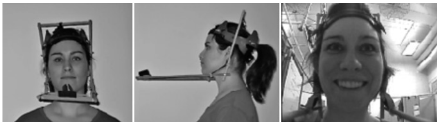
Fig. 12.1 Head mount apparatus used to support video camera for recording facial expression. The adjustable mount for the camera is located at the tip of the horizontal strut. The right photo is the face view captured from the head-mounted camera
