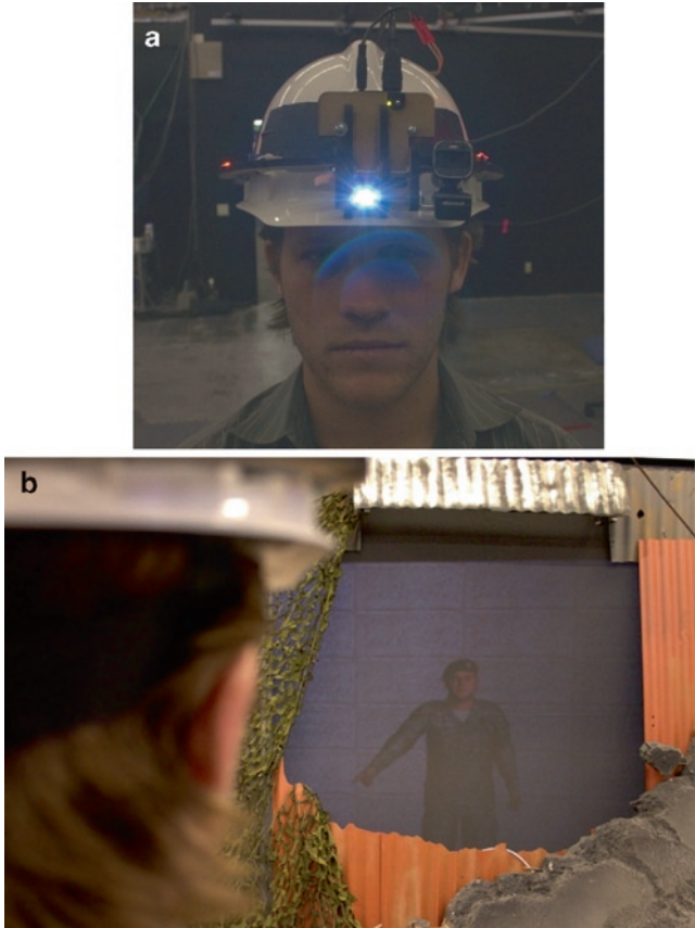
Fig. 5.4 (a, b) The REFLECT head mounted projector and associated projected imagery
