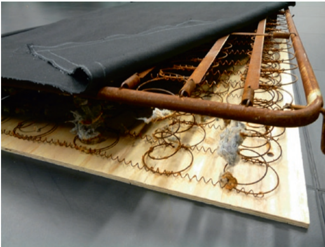
Fig. 2.2 Springboard input platform made from a crib spring, a board and black cloth
