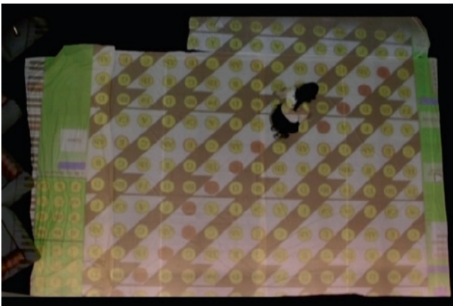
Fig. 3.3 An earlier whole body version of Harmony Space designed to use floor projection and camera tracking
