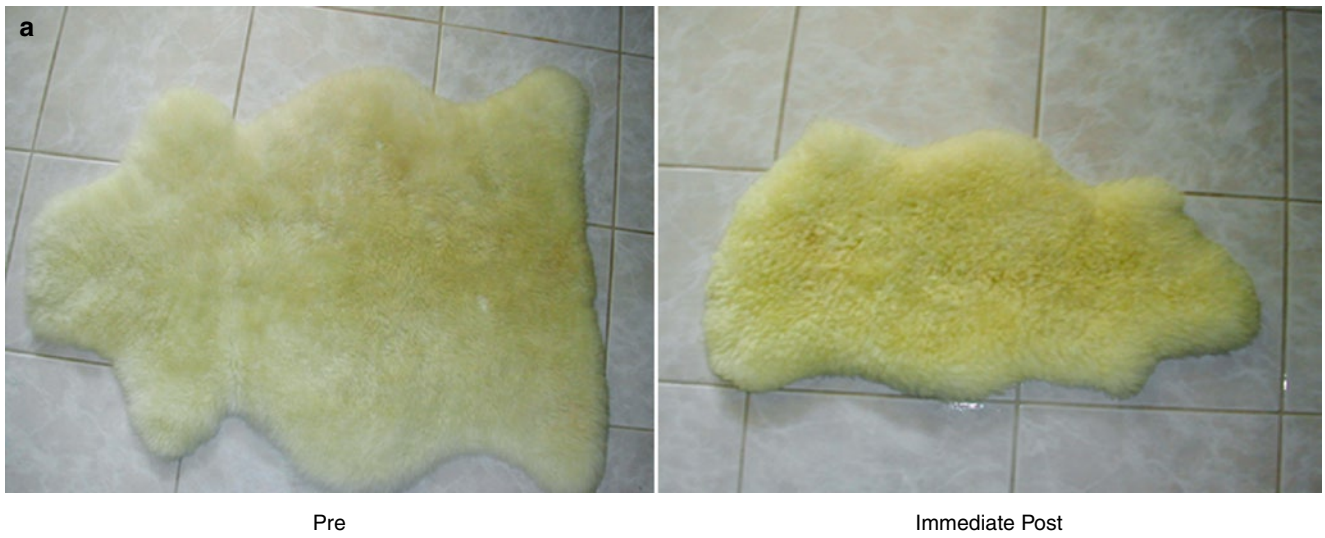
Fig. 12 (a, b) Animal hide contraction with slow sustained heat
