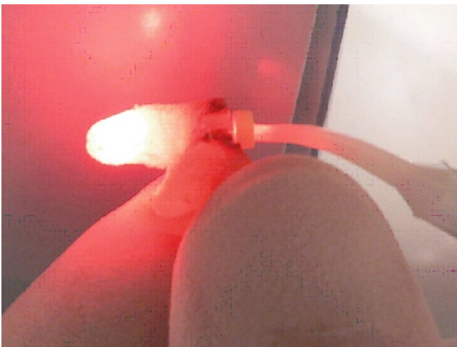
Fig. 34 320 µm diameter quartz optic fibre inserted into a root canal. The red aiming beam shows the extent of light distribution that might be expected with IR laser energy
