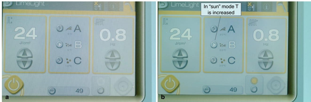
Fig. 6 Figure shows user controllable temperature change with an IPL. By increasing the handpiece tip temperature, pigmented lesion heating is favored over vascular heating
