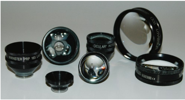
Fig. 6 Commonly employed ophthalmic lenses. A multitude of lenses can be used for argon laser treatment application depending on the desired magnification and field of view. Such lenses can be broadly categorized as either corneal contact lenses (five lenses located on the left: ocular Mainster 165, ocular three mirror, ocular Yannuzzi fundus, ocular Reichel-Mainster and ocular Mainster wide field) or indirect lenses (two lenses located on the right: 20-diopter and 28-diopter)
