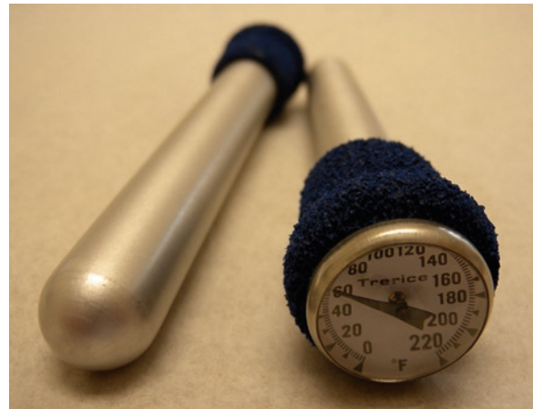
Fig. 21.4 Calymetric metal cylinders used for evaluation of temperature sensation recovery
