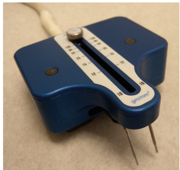
Fig. 21.2 PSSD device with two blunt prongs with adjustable interprong distance
