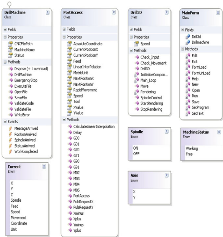
Fig. 5.14 UML static diagram of drill project
