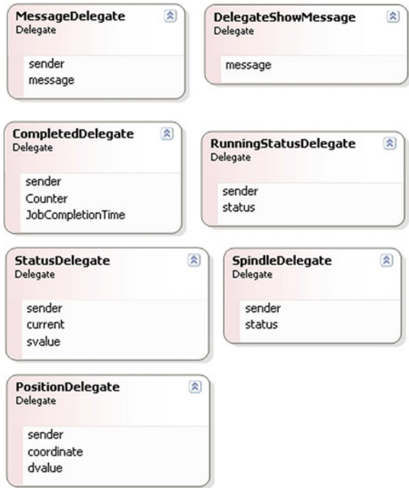
Fig. 11.68 UML Static Structure of VirtualFactory. VirtualFactoryLib Delegates
