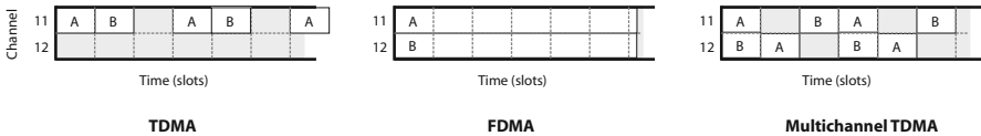
Fig. 2.6 TDMA, FDMA and multi-channel TDMA for two transmitters (A and B) on 802.15.4-channels 11 and 12 in the ISM band
