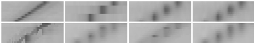
Fig. 10 Edges from a trench between two regions of similar intensity from an image of annealed gold, subsampling by 4 in the vertical direction. Left to right, top to bottom : Original image; nearest neighbor interpolation; bicubic interpolation; contour stencil interpolation; PLI; H1 inpainting; TV inpainting; LCIS inpainting
