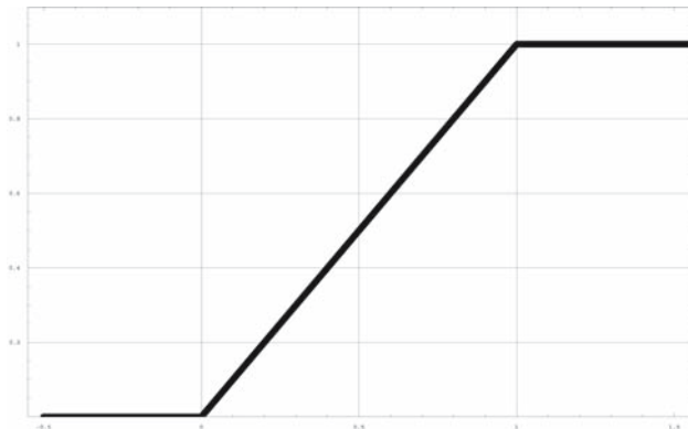
Fig. 7.2.1. The dependence of the optimal signal-to-noise ratio on the detection time t_0 for the matching filter from Example 7.2.1. The input signal is the sum of a rectangular signal of amplitude A = 1 , duration T = 1 , and the white noise with autocorrelation function \gamma_N(t) = \delta(t) .
