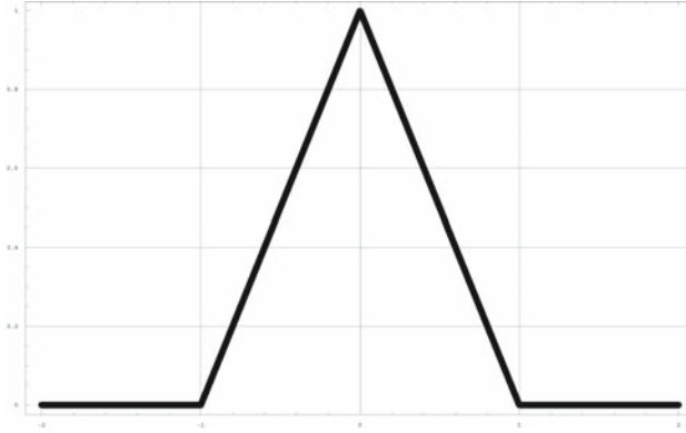
Fig. 6.1.2. The output autocorrelation function \gamma_Y(\tau) (6.1.10) of the integrating system (6.1.8) with T = 1 , in the case of the standard white noise input X(t) = W(t) .
