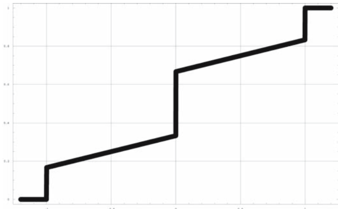
Fig. 3.1.7. Cumulative distribution function (c.d.f.) F_X(x) of mixed type described by formula (3.1.10). This distribution has both discrete and continuous components.
