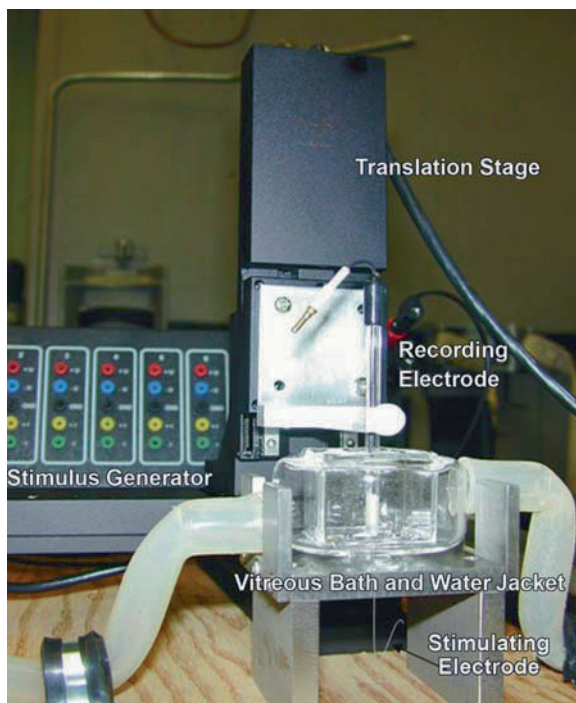
Fig. 9 Apparatus for automated field potential measurements. Positioning was achieved with a computerized Thorlabs XYZ translation stage. The recording electrode was attached to the stage hardware and controlled by the computer. Stage movement was programmable so that any position could be reached with mouse a click away from the experimental set up to minimize human intervention
