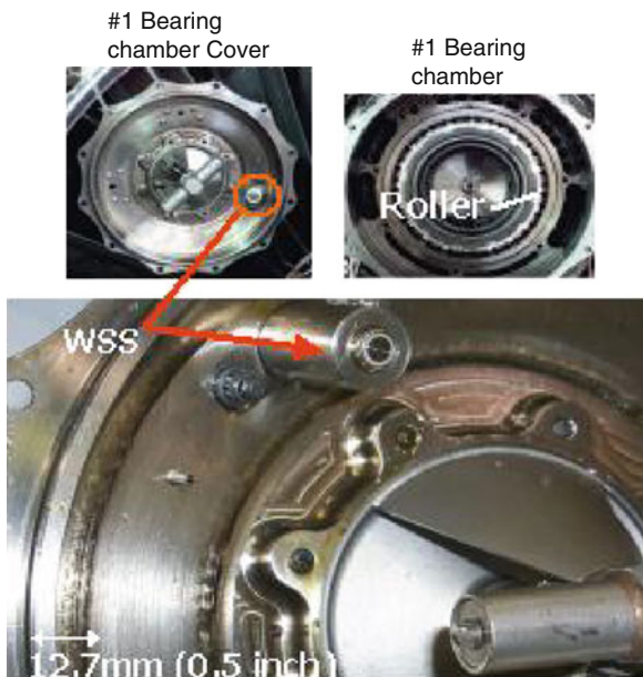
Bearing Wear Monitoring Using Electrostatic Charge, Fig. 4 Wear-site sensor location in F100 seeded fault engine tests, conducted by Pratt and Whitney. Four electrostatic sensors were installed in the oil system of the F100 engine to monitor bearings #1 and #5 seeded fault engine test (Powrie et al. 1999c, 2000)
