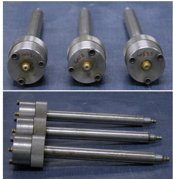
Bearing Wear Monitoring Using Electrostatic Charge, Fig. 5 Electrostatic Wear-Site Sensors (WSS) used in bearing test facility at University of Southampton
