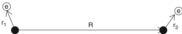
Basic Concepts in Adhesion Science, Fig. 1 Schematic diagram of two hydrogen atoms separated by a distance large compared to the Bohr radius but close compared to the mean spacing in an ideal gas
