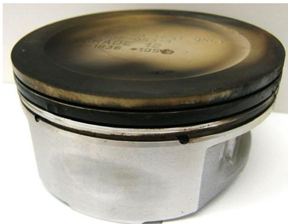
**Additive Chemistry Testing Methods, Fig. 1** Deposits formed on pistons during ASTM D7320 engine test
