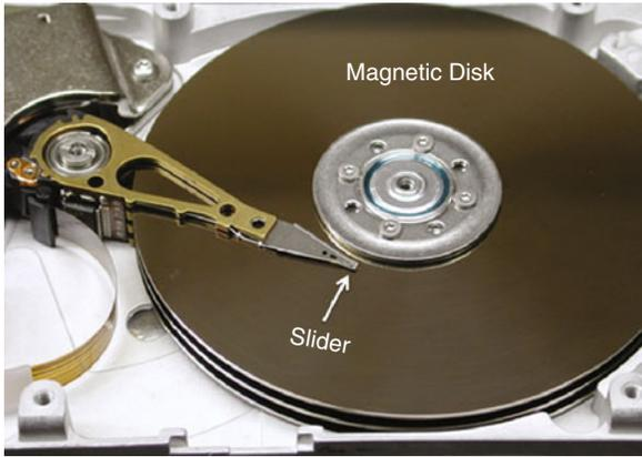
**Applications of DLC in Magnetic Recording, Fig. 7**
