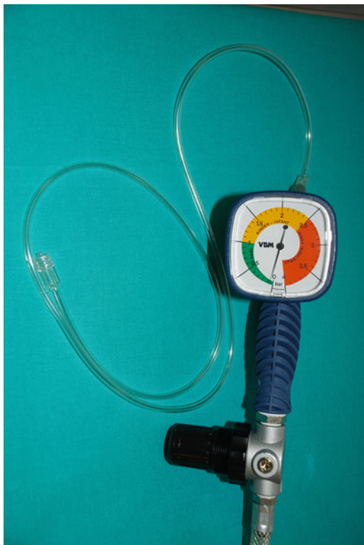
Figure 13.11. Manujet injector. Large-bore tubing for conducting gas from the source to the injector, pressure regulator, handle with trigger and manometer, and small-bore tubing for conducting gas from the injector to the catheter.
