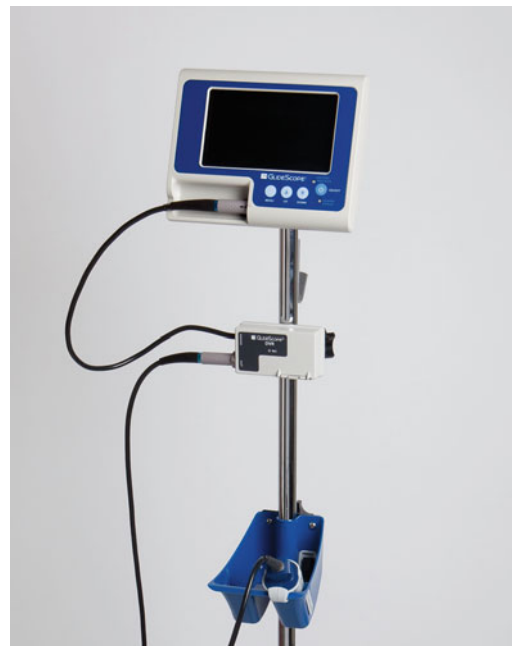
Figure 6.13. A GlideScope digital video recorder (DVR) has been connected between the laryngoscope and the monitor. When the monitor is powered on, recordings are automatically saved to a Secure Digital (SD) flash drive and time stamped. Used with permission, ©Verathon Inc.
