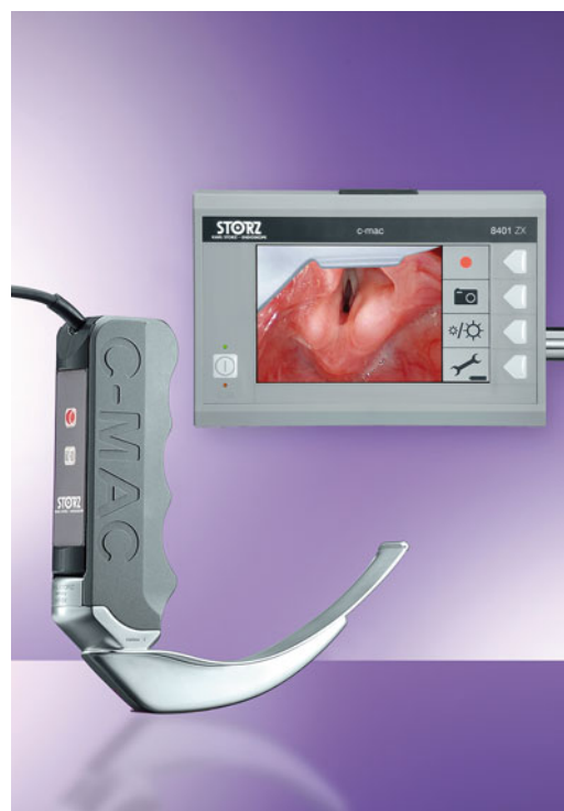
Figure 6.27 The third-generation Storz VL is the C-MAC which employs video chip (CMOS) technology. The camera is located distally and the image is displayed on a dedicated battery-operated monitor with on-board recording of still (jpeg) or video images (mpeg). Recordings can be initiated on the monitor or the handle itself. © 2011 Photo courtesy of Karl Storz Endoscopy-America, Inc.
