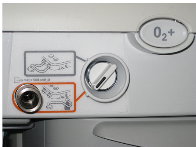
Figure 13.8. Anesthesia-machine flush valve of the Datex-Ohmeda S/5 Avance. Note that the maximum pressure is less than 1 atm.
