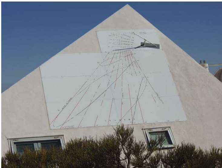
Fig. 5.19. A sundial placed on an inclined wall at the Teide Observatory (Tenerife), based on a design by Mario Salomone.
