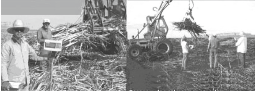
Fig. 6 Quick measurement of total culm weight of a plot in FT7 using a wireless controlled dynamometer
