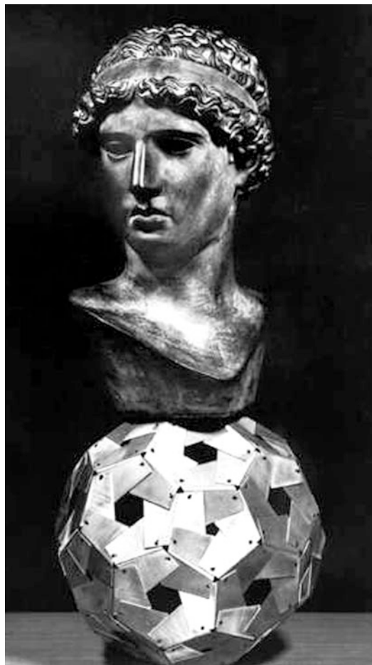
Figure 12.23. A mechanical model illustrating rigidity in a T = 3 icosahedral lattice, built of 90 identical pieces of \frac{1}{32} -inch-thick sheet aluminum bent to represent dimers connected by pentamer/hexamer bonds. The diameter along the threefold axis is 11.5 inches, and the model weighs 2 pounds. Its shape approximates a truncated Platonic icosahedron, and it supports without distortion a 32-pound plaster bust of Plato.
