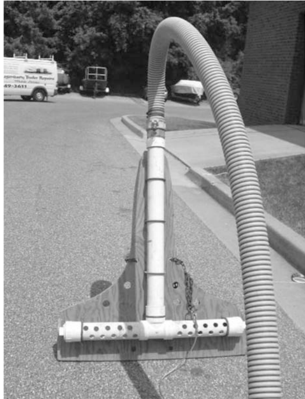
Fig. 1 Detail of the underside of the suction-dredge head and plywood delta wing
