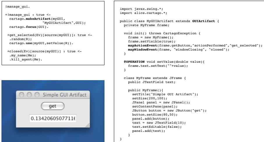
Fig. 8.13 An example of simple GUI artifact implementation (right) used by a Jason agent (top-left).
