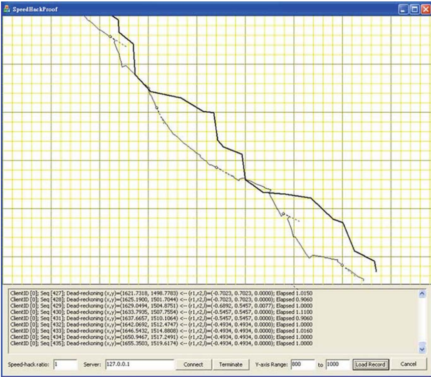
Fig. 16 The path of the local avatar Q ( thicker line ) and the path of the non-local avatar \mathcal{P} ( thinner line ) rendered on Q 's local machine which zoomed into the last 60 s
