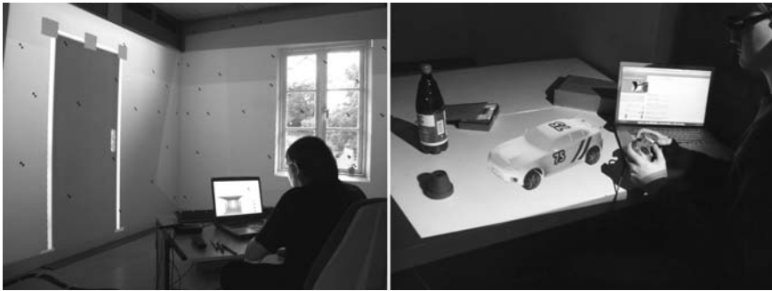
Fig. 4 Examples for spatial augmented reality applications with projector camera systems. An immersive in-place visualization of an architectural lighting simulation (left), and a stereoscopically projected spatial augmented reality game (right). Door, window, illumination and the car are projected
