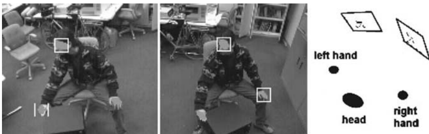
Fig. 6 3D tracking of user's hands and head, view from the left and right camera
