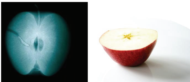
Fig. 5.6 X-ray and classic view of an apple. X-ray can be useful for detecting internal defects without slicing the fruit.
