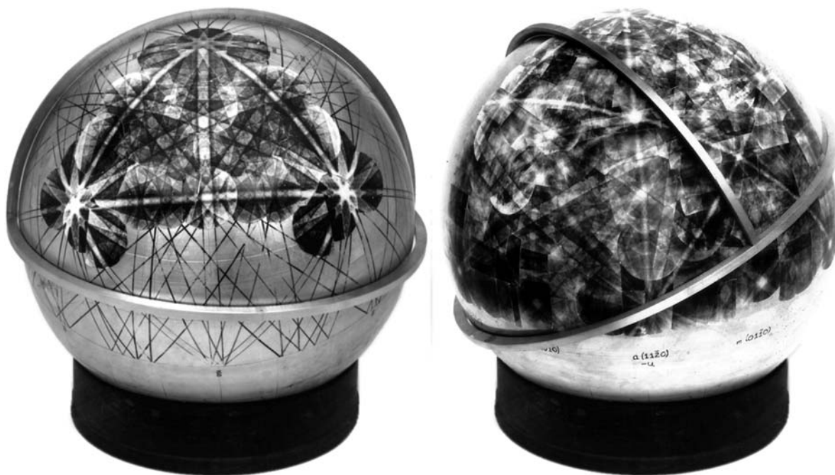
Fig. 5.2 Spherical Kikuchi maps for ferrite (left, courtesy of Bevis Hutchinson) and quartz (courtesy of Geoff Lloyd). The composite ECPs cover 1/24 th (ferrite) and 1/6 th (quartz) of the spherical surface. For the ferrite, the four-fold \langle 001 \rangle zone can
