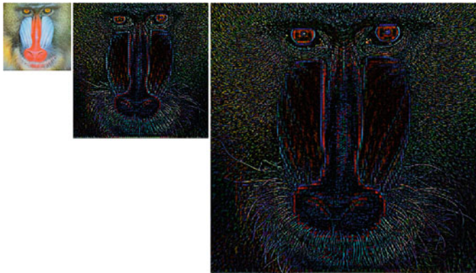
Fig. 9.8 Multiscale representation of the baboon image. Left: The coarsest level image \mathcal{I}_2 . Middle: The residual image \mathcal{I}'_1 . Right: The residual image \mathcal{I}'_0 . The data at each level are modeled by the hybrid linear models. The contrast of the middle and right images has been adjusted so that they are visible.
