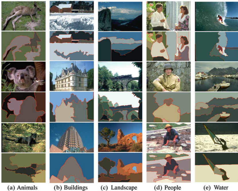
Fig. 10.8 Representative segmentation results (in color) of the TBES algorithm on various image categories from BSD. For each image pair, the top is the original input image, and the bottom is the segmentation result, where each texture region is rendered by its mean color. The distortion \varepsilon was chosen adaptively to optimize PRI.
