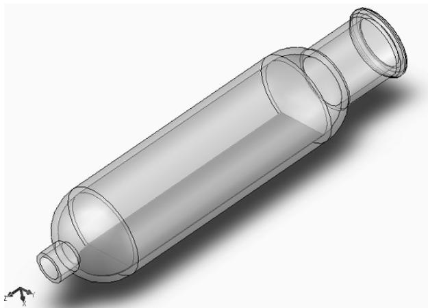
**Figure 1.** Diagram of the thin film rotating tonometer.
