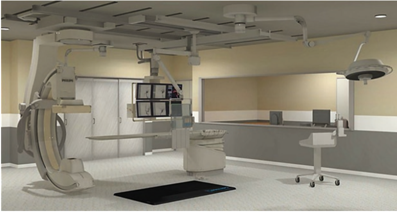
Fig. 12.5 Artist rendition of a hybrid operating room with interventional capabilities. A separate shielded booth allows for remote fluorography, limiting operator radiation exposure (Courtesy of Koninklijke Philips Electronics)
