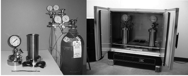
Figure 2—Pressure cell and forced air oven used for the high pressure incubation.
