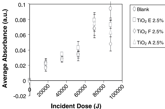
Figure 28—Extent of UV degradation in the epoxy system as monitored by ATR-FTIR. An increase in the oxidation products is shown by the C=O stretch at 1762\text{ cm}^{-1} for epoxy films with TiO 2 F (diamond), with TiO 2 E (square), and with TiO 2 A (triangle). Error bars represent the estimated uncertainty of K=2 (95%).
