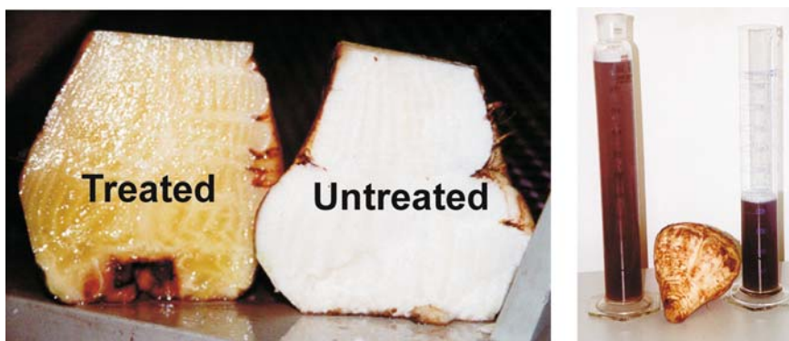
Fig. 14 Cut through sugar beets before and after treatment in the reaction chamber together with the corresponding yield of juice obtained by cold pressing with 32 bar pressure for 15 minutes
