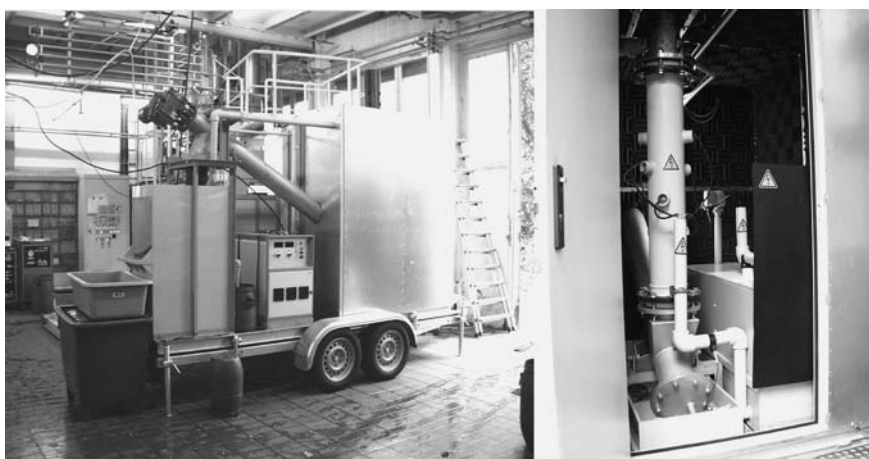
Fig. 13 The mobile test device KEA used to demonstrate the potential advantages of electroporation for the production of sugar from sugar beets. The left part shows the complete set up. The photo on the right depicts the treatment vessel
