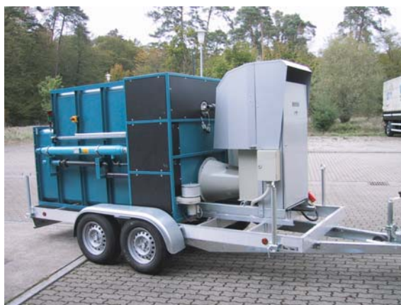
Fig. 19 Mobile facility KEA-Wein for the treatment of grape mash with strong PEFs
