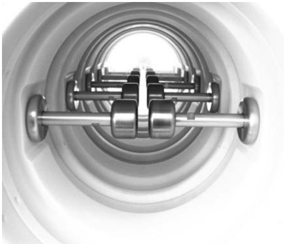
Fig. 4 Set of spark gap switches with Borda electrode profiles in a common switch housing
