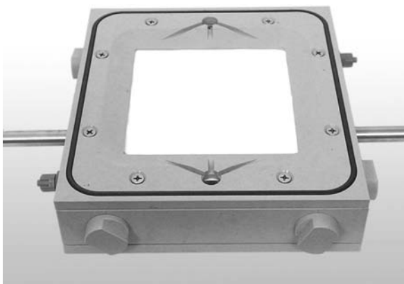
Fig. 9 Filter chamber of the electrofilter plate SYMBIOSE250
