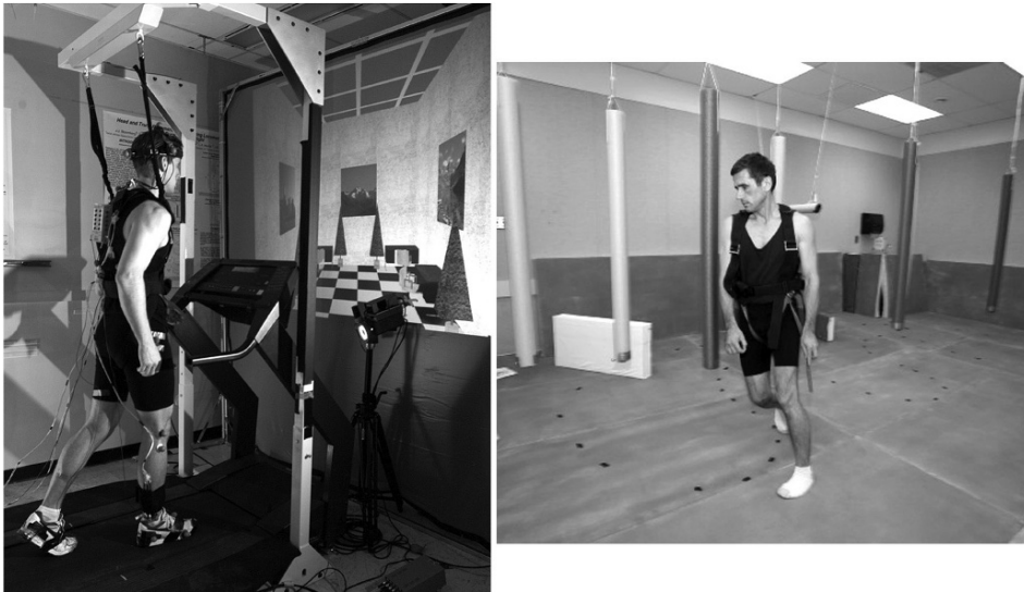
Figure 5-11. Left. While subjects walk at 6.4 km/h on a motorized treadmill, three-dimensional full-body motion data are acquired using a video-based motion analysis system; gait cycle timing is measured using foot switches placed in the shoes and dynamic visual acuity is assessed. Right. The Functional Mobility Test provides an assessment of the functional and operational changes in locomotor function by testing subject's ability to negotiate an obstacle course over a medium-density foam floor. Photos courtesy of NASA.
