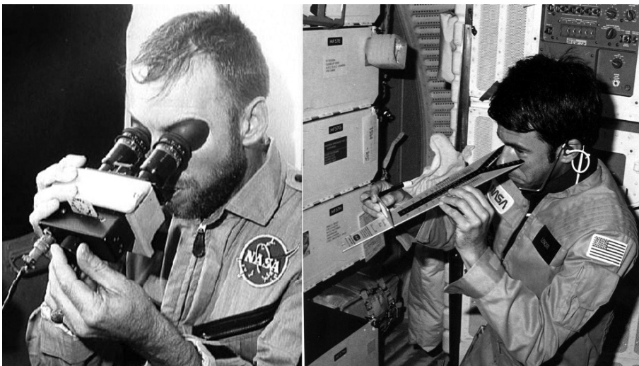
Figure 4-03. Left. The visual acuity of the Gemini-5 and 7 crew was tested each day using an in-flight vision tester, which was a binocular optical device containing a transilluminated array of 36 high-contrast and low-contrast rectangles. Half of the rectangles were oriented vertically in the field of view, and half were oriented horizontally. The flight crew made forced-choice judgments of the orientation of each rectangle and indicated their responses by punching holes in a record card. No significant difference was noted between preflight and in-flight measurements. Right. No significant differences in diopter measurements were measured neither in the near point of accommodation (near-vision acuity) among the pre-, in-, and postflight conditions in 23 crewmembers of the Space Shuttle. Photos courtesy of NASA.
