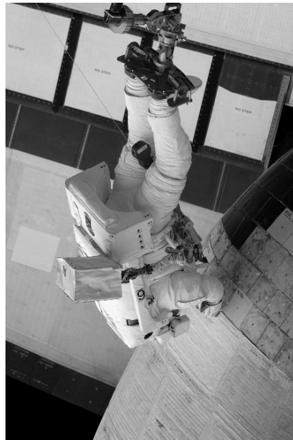
Figure 9-06. During an extra-vehicular activity, an astronaut hanging “upside-down” at the end of the remotely-operated robotic arm is inspecting the insulating tiles of the Space Shuttle. Episodes of height vertigo have been reported during unfamiliar visual orientations. Photo courtesy of NASA.
