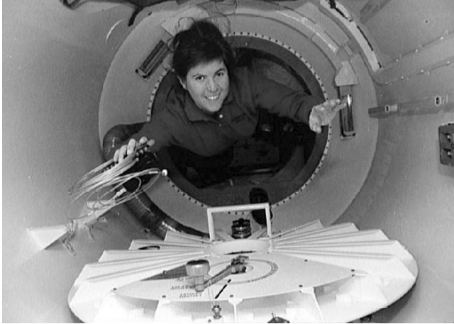
Figure 3-03. Astronauts often complained that going through the tunnel connecting the Space Shuttle middeck and the Spacelab module was particularly disorienting and provocative of space motion sickness symptoms. Photo courtesy of NASA.
