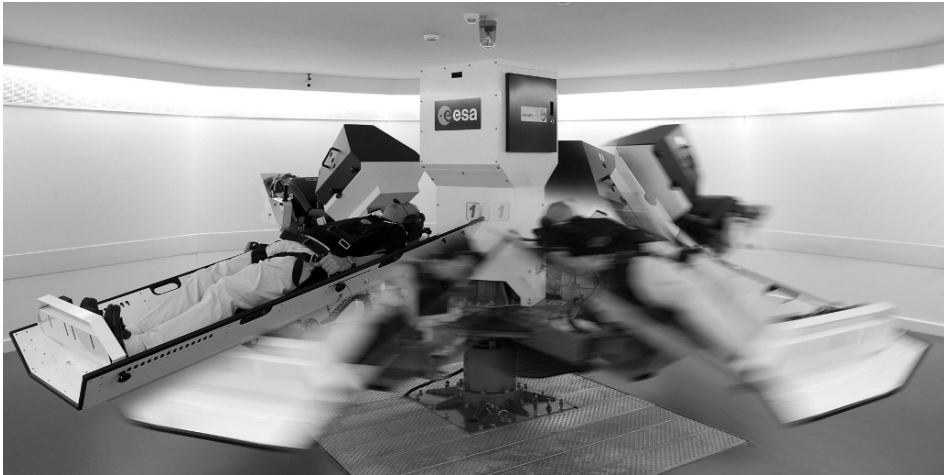
Figure 8-13. Artificial gravity is being tested during bed rest by spinning volunteers on a short-radius centrifuge. Because of the deconditioning that takes place during bed rest, subjects after bed rest typically experience orthostatism intolerance when moving from lying down to standing upright. Prescriptions including intermittent spinning on the centrifuge (1 hour/day with 1 g at the heart level) were shown to be effective against this deconditioning. This photograph shows the ESA short-radius centrifuge utilized during bed rest studies at MEDES in Toulouse. Photo courtesy of CNRS/Sébastien Godefroy.
