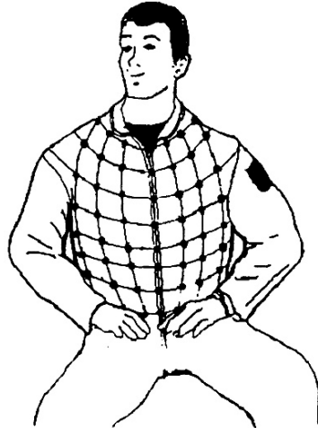
Figure 3-09. Researchers at the Naval Aerospace Medical Research Laboratory (NAMRL) in Pensacola (Florida) have developed the Tactile Situation-Awareness System (TSAS), which uses the sense of touch to provide spatial orientation and situational awareness information to aviators. The system could be applied to astronauts during teleoperation tasks or extra-vehicular activity.
