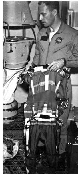
Figure 5-02. One of the engineering and technology experiments on board Skylab was a special suit instrumented to measure body motions as the wearer went through typical tasks on board the space station. One Skylab astronaut inspects such a vest during a training session on Earth. Photo courtesy of NASA.
