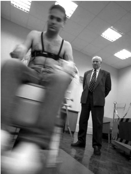
Figure 8-03. Cosmonaut vestibular training at Star City in Moscow, Russia. During passive rotation in yaw the cosmonauts tilt their head in pitch and in roll until they develop symptoms of motion sickness. These sessions are required daily during the last couple of weeks prior to a space flight on board the Soyuz vehicle. Photo courtesy of CNES.
