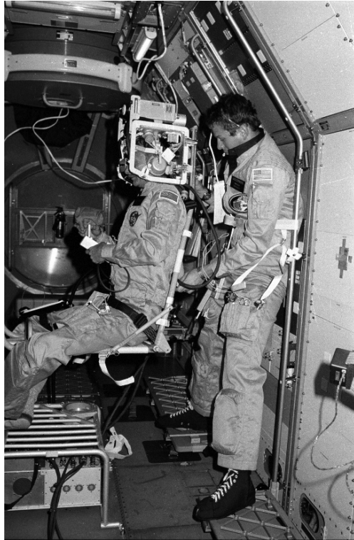
Figure 4-17. The Body Restraint System (BRS) flown on board the first Spacelab mission was used to evaluate changes in the threshold of perception of linear acceleration during adaptation to microgravity. An operator manually moved the BRS, while the subject reported the beginning and direction of perceived motion using a joystick. Photo courtesy of NASA.
