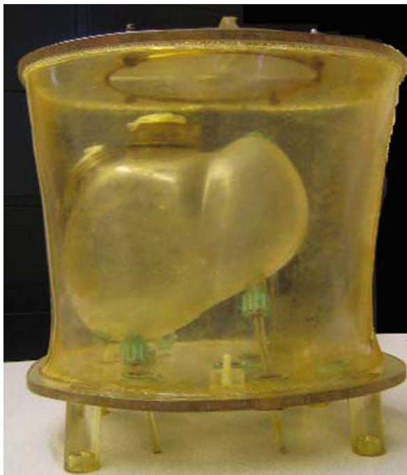
**Fig. 15.5** A phantom of the human torso with two chambers – outer chamber corresponding to an adult torso, and inner chamber corresponding to an adult human liver. Both chambers can be filled separately with any desired material.
