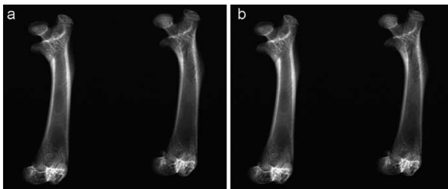
Fig. 14.6 Images made by 40-keV X-ray radiography of (a) calcified bones (i.e., heated at 600°C for 5 h) and (b) natural bones. The distinction between the cortical (surface) and the trabecular (inner) bone regions is evident [18]
