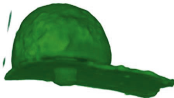
Fig. 13.13 Neutron tomography from bronzes [44] provided information on the spatial distribution of the components forming the samples. Measurements were performed at the Cold Neutron RADiography (CONRAD) instrument at the Hahn-Meitner Institut (Berlin, Germany)
