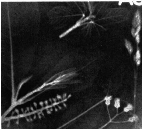
Fig. 14.1 Neutron radiography of plant tissues demonstrates the sensitivity of neutrons to hydrogenous materials [3]
