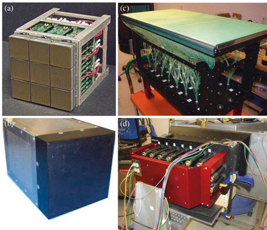
Fig. 4.3 (a) The figure shows an optical detector assembly of an Anger camera module for the SNAP high pressure diffractometer at the Spallation Neutron Source (SNS) at Oak Ridge National Laboratory. Nine 8 \times 8 channel position-sensitive photomultiplier tubes are assembled to form a single Anger module. (b) A SNAP module is shown with the bezel, which contains a 15 cm square {}^6\text{Li} glass scintillator. This detector has a two-dimensional position resolution of 1.3 mm full width at half maximum (FWHM). (c) A crossed wavelength-shifting fiber assembly for a detector module to be mounted on the Vulcan engineering diffractometer at SNS is shown. The wavelength-shifting fibers collect the blue scintillation light from a {}^6\text{LiF}/\text{ZnS}(\text{Ag}) scintillator screen and guide the shifted green light to a coded photomultiplier array. (d) A completed Vulcan module operates for initial calibration. This 80 \text{ cm} \times 40 \text{ cm} detector module has 5 mm wide by 37.5 mm tall pixels, with resolution matched to the diffractometer
