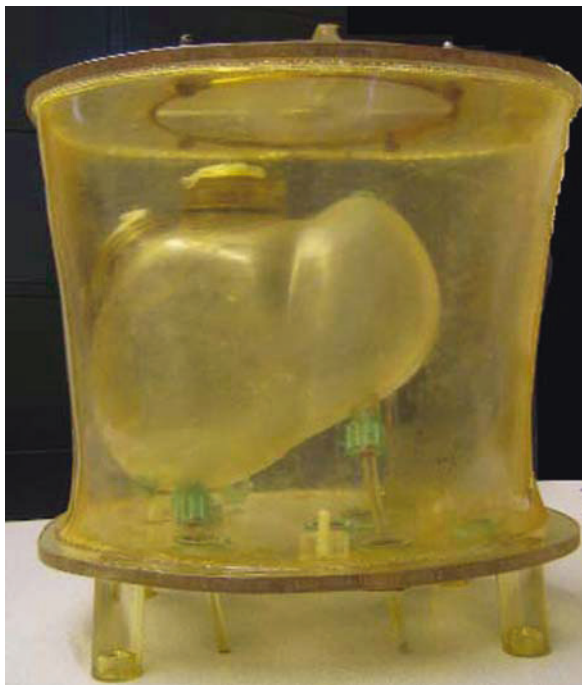
Fig. 15.5 A phantom of the human torso with two chambers – outer chamber corresponding to an adult torso, and inner chamber corresponding to an adult human liver. Both chambers can be filled separately with any desired material. (Figure from Kapadia et al. [32], pp. 2633–2649. © Institute of Physics and IOP Publishing Limited 2008)
