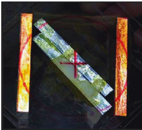
Fig. 15.2 Geometry of the phantom imaged in the tomography experiment. The vertical outer bars represent copper while the diagonal inner (gray) bars represent iron. Each bar measures 0.6 cm by 6 cm by 2.5 cm.
