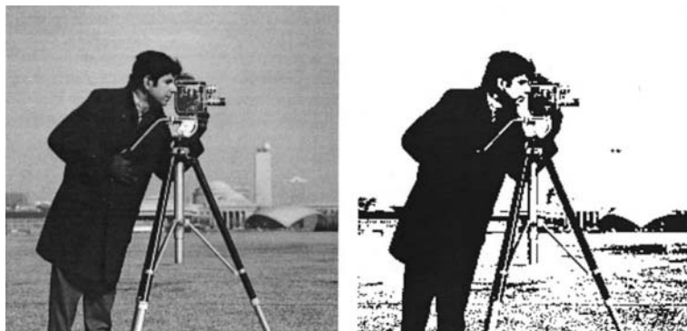
Image Data Representations. Figure 1. (a) A monochrome image (b) Its binary equivalent.
