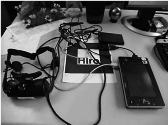
Interactive Virtual Humans in Mobile Augmented Reality. Figure 6. A wearable UMPC with the i-glasses HMD, battery pack and usb webcam.
