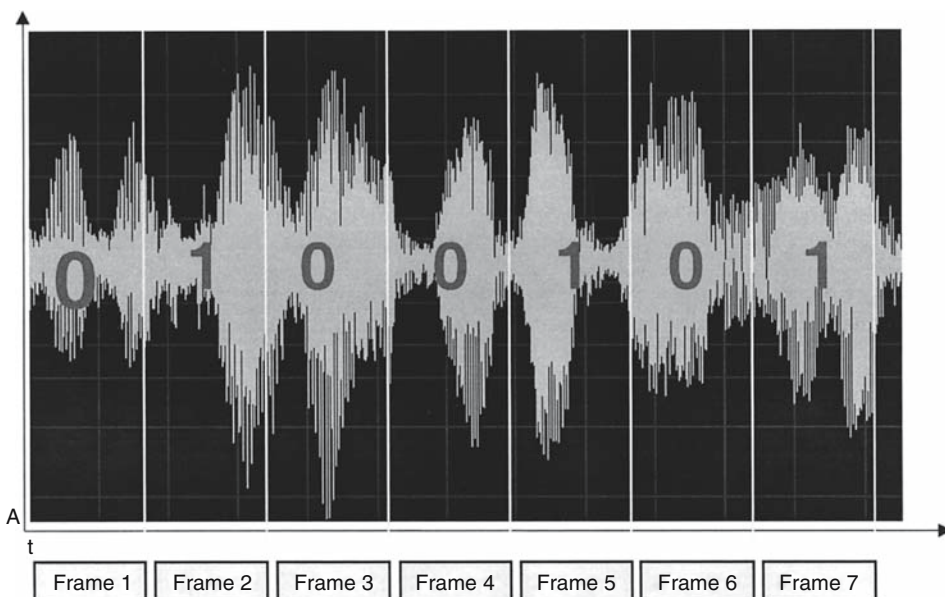
Watermarking, Audio. Figure 1. Audio watermarking usually embeds single bits in discrete time frames.
