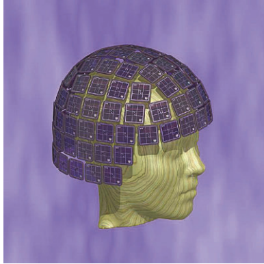
FIGURE 15.3. Helmet-shaped device with array of sensors uniformly distributed around the head to provide MEG measurements. Source: l1l.tkk.fi/research/brain/head.jpg
