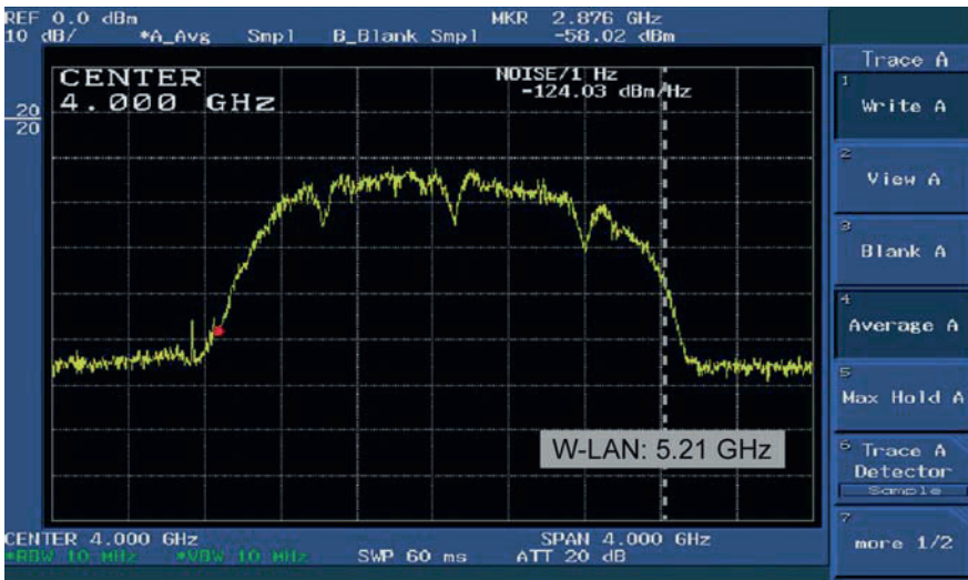
Fig. 3 Spectra of DS-UWB and wireless LAN
