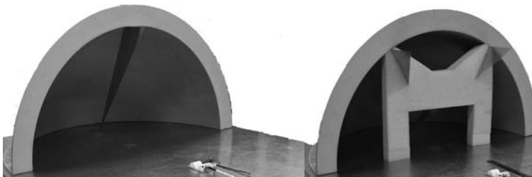
Fig. 2 Experimental setups for two-feed arm and 60° four-feed arm prolate-spheroidal IRA
