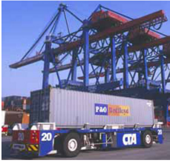
(a) AGV in front of quay cranes (courtesy of HHLA).
