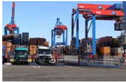
(b) Trucks (DRMG on the right; quay cranes in the background) (courtesy of HHLA).
