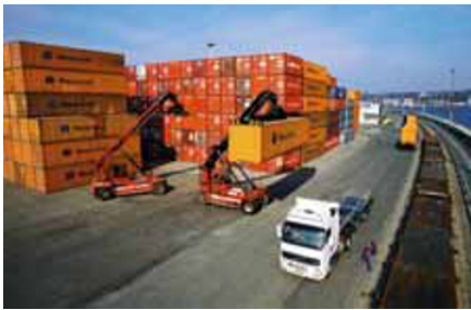
(a) Reachstackers and trucks (courtesy of HHLA).
