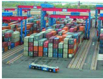
(b) DRMG with an AGV in front (courtesy of HHLA).
