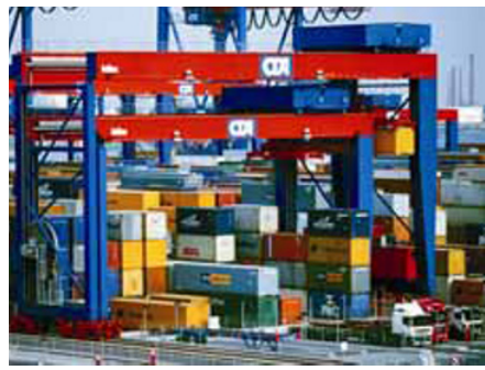
(b) Stacking cranes (here: DRMG) serving a container block in the yard (courtesy of HHLA).
