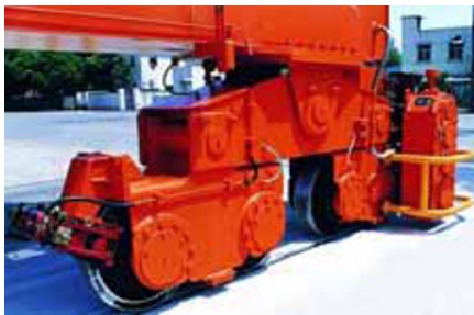
(a) Wheel of a RMG on rail (courtesy of Shanghai Zhenhua Port Machinery – ZPMC, www.zpmc.com ).
