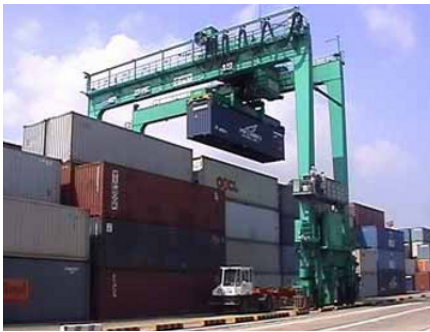
(a) RTG beneath a block serving an internal truck (courtesy of ZPMC).
