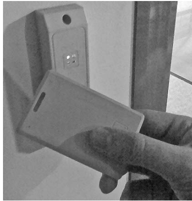
Fig. 2.5 Card door access. A camera at the door takes a photo and compares it to the facial template stored on the card to determine whether or not to allow access.
