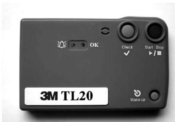
Fig. 5.7 A continuous monitoring device for measuring and recording temperatures of a food storage environment
