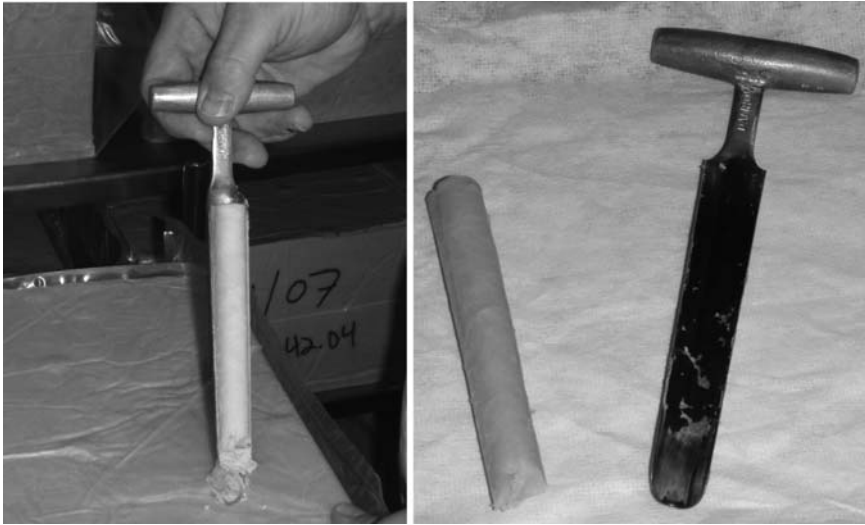
Fig. 9.4 Removing a cheese plug from a 40-lb block with a 127 mm (5-in) trier
