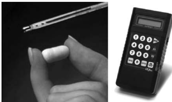
Fig. 5.8 A wireless “temperature pill” and data recorder for continuous measurement of the internal temperature of a milk container
