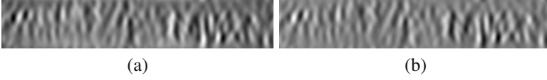
Fig. 4.16 Real and imaginary outputs of convolving an image with a 2D Gabor wavelet.
