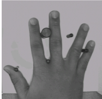
Fig. 5.9 Example showing incorrect placement of the hand in a peg-based system..
