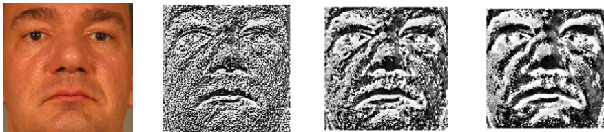
Fig. 3.30 Local Binary Pattern (LBP) images encoded at different scales. From left to right: original image; images encoded using LBP_{8,1} , LBP_{8,3} , and LBP_{8,5} operators, respectively.
