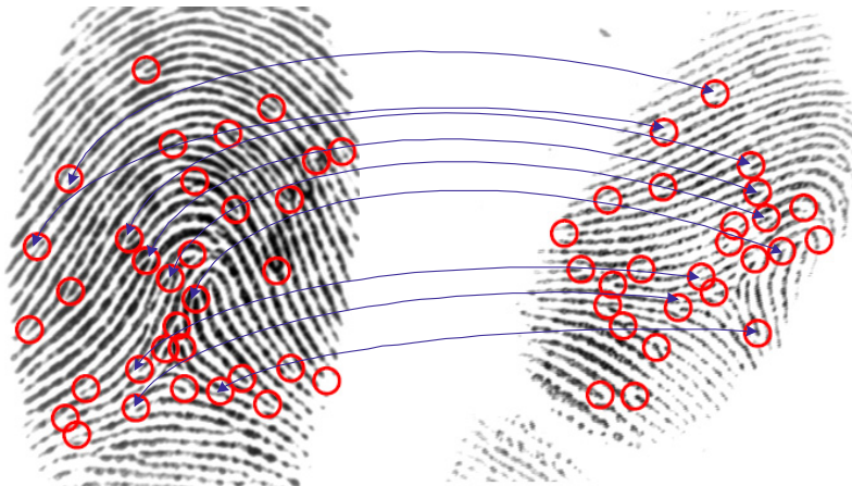
Fig. 1.9 Illustration of intra-user variability in fingerprints. Two different impressions of the same finger obtained on different days are shown with minutiae points marked on them. Due to differences in finger placement and distortion introduced by finger pressure variations, the number and location of minutiae in the two images are different (33 and 26 in the left and right images, respectively). The number of corresponding/matching minutiae in the two images is only 16. Some of these correspondences have been indicated in the figure. The concept of minutiae points will be described in the next chapter.
