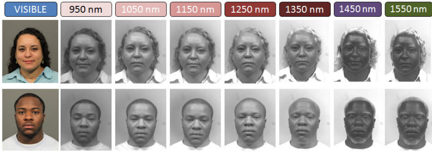
Fig. 3.8 Face images captured in the visible and near-infrared spectra at different wavelengths.
