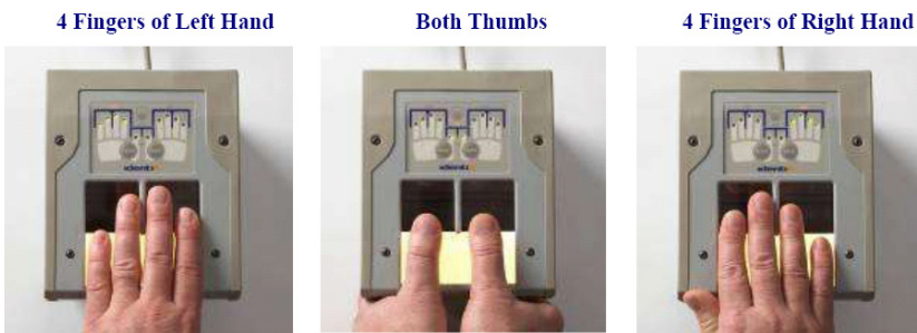
Fig. 6.6 A fingerprint sensor developed by Identix that allows rapid acquisition of all ten fingers in three steps. (Source: Nationwide Solutions)
