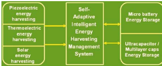
Fig. 1.26 Schematic of the architecture required for self-powered wireless sensor network to achieve desired reliability for long period of time
