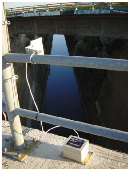
Fig. 7.7 Solar-powered wireless G-Link ® seismic sensors on Corinth Bridge, Greece
