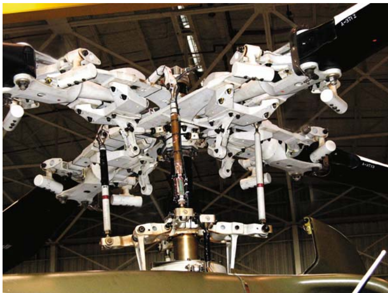
Fig. 7.3 Pitch-Link Installed on Bell 412 Helicopter
