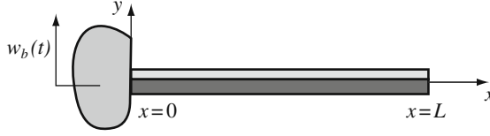
Fig. 2.2 Cantilevered beam excited by the motion of its base in the transverse direction
