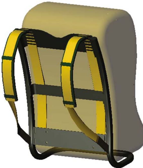
Fig. 17.12 Schematic of the backpack with piezoelectric straps
