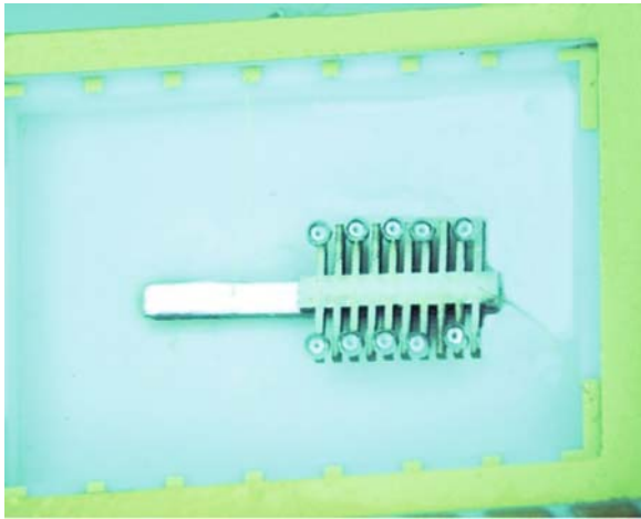
Fig. 1.7 Assembled energy harvesting device using laser micromachining (Copyright: IEEE)
