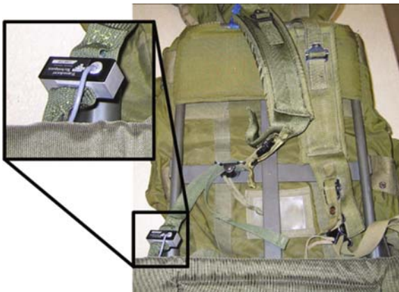
Fig. 17.6 Instrumented backpack used to experimentally determine the loading in the straps
