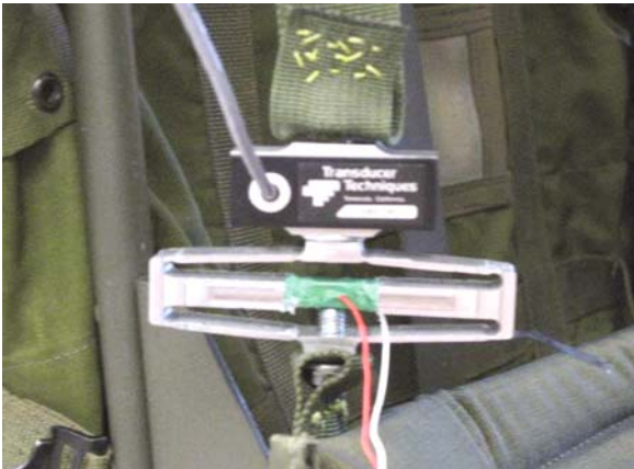
Fig. 17.23 Stack amplifier installed in series with a force transducer for simultaneous measurement of force and voltage
