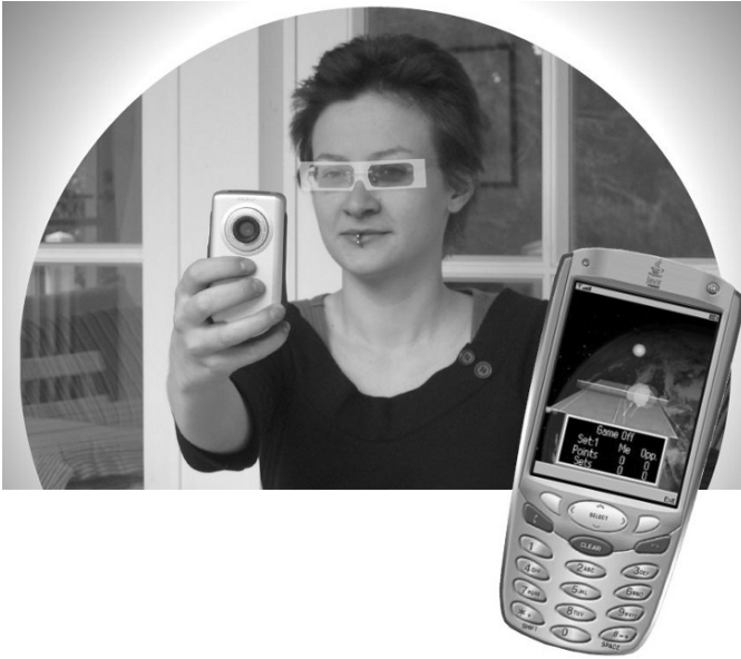
Fig. 15.2. Symball virtual table tennis game on camera phones[193], using StereoGames software [576] to create depth illusion.
