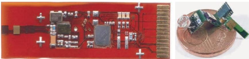
Fig. 9.11 Examples of functional layer technology (sensor nodes)
