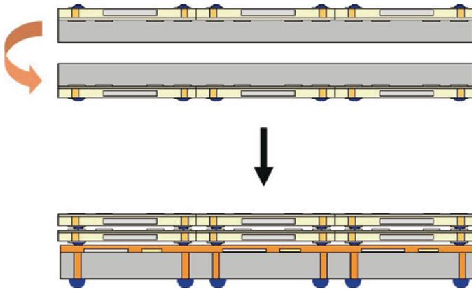
Fig. 9.10 Principle of the functional layer technology
