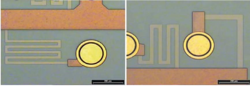
**Fig. 9.7** Integration of resistors into a wafer-level package
