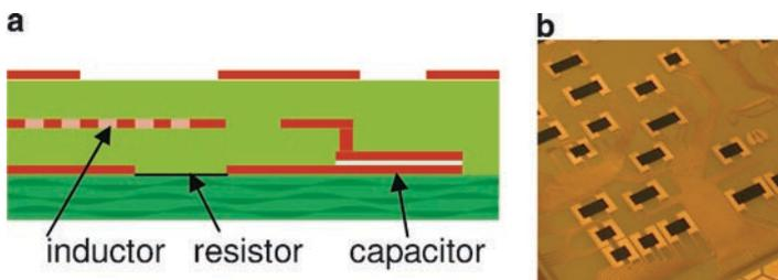
**Fig. 9.13** (a) Embedded inductor, resistor, and capacitor in the build-up layers of a printed wiring board; (b) Printed resistors on a flexible printed wiring board before lamination into a build-up layer
