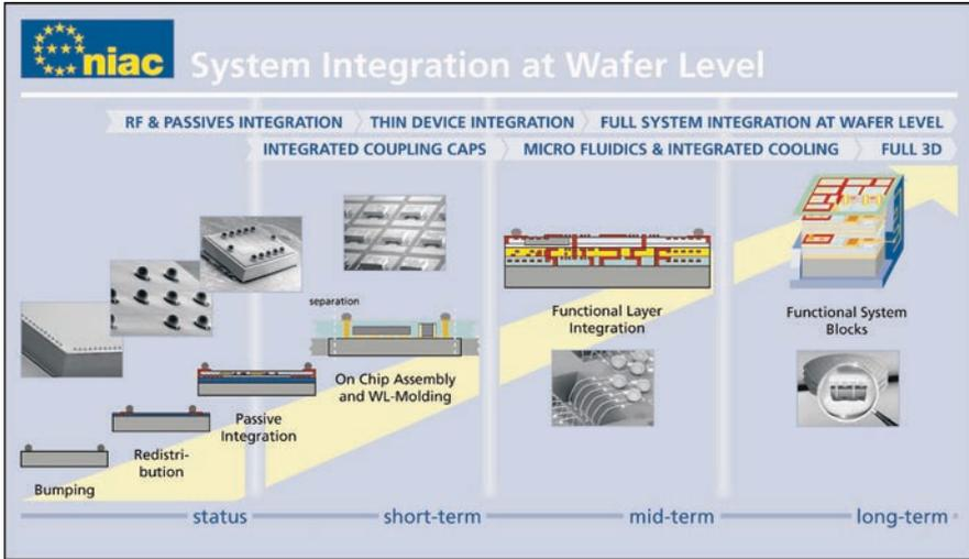
Fig. 9.4 Technology roadmap: wafer-level system packaging [8]
