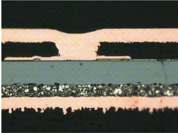
using local fiducials for die placement, laser drilling, and laser direct imaging. Figure 9.15 shows a cross section of a Cu interconnect to an embedded chip.
