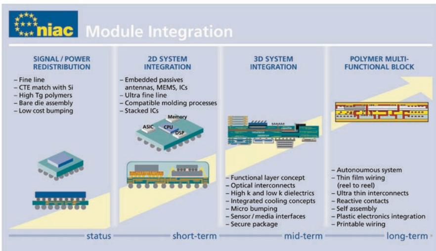
Fig. 9.12 Technology roadmap for module level system integration [8]
