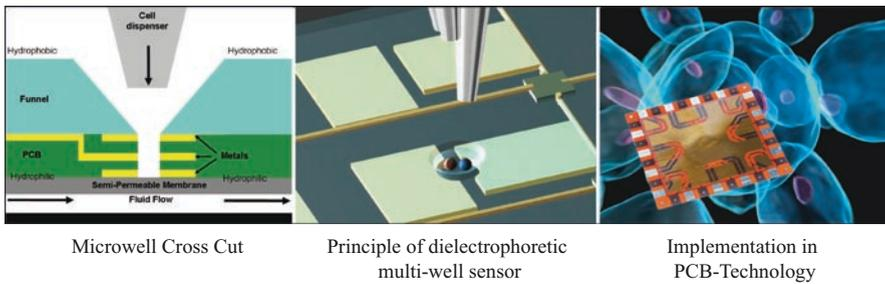
Fig. 9.18 Using PCB technologies for lab on substrate [19]
