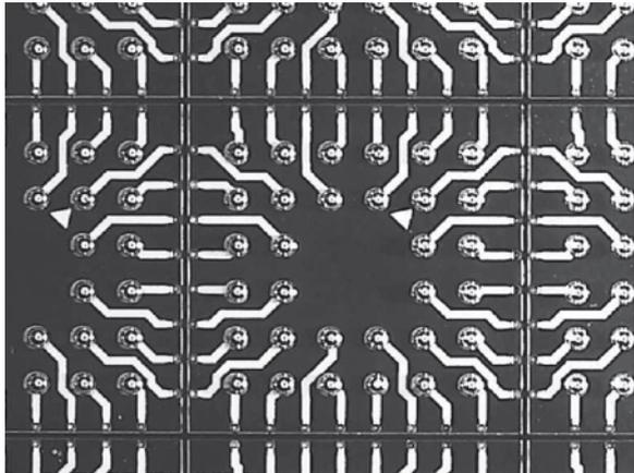
be preferred. A highly specialized plasma etching process is used to structure the silicon. Preferably, tapered side walls are used for all structures. The deposition of dielectric layers over the silicon guarantees electrical isolation during the subsequent redistribution process, which is based on polymer/Cu or Al. After UBM deposition, the wafer is ready for the balling and dicing process (Fig. 9.26).
